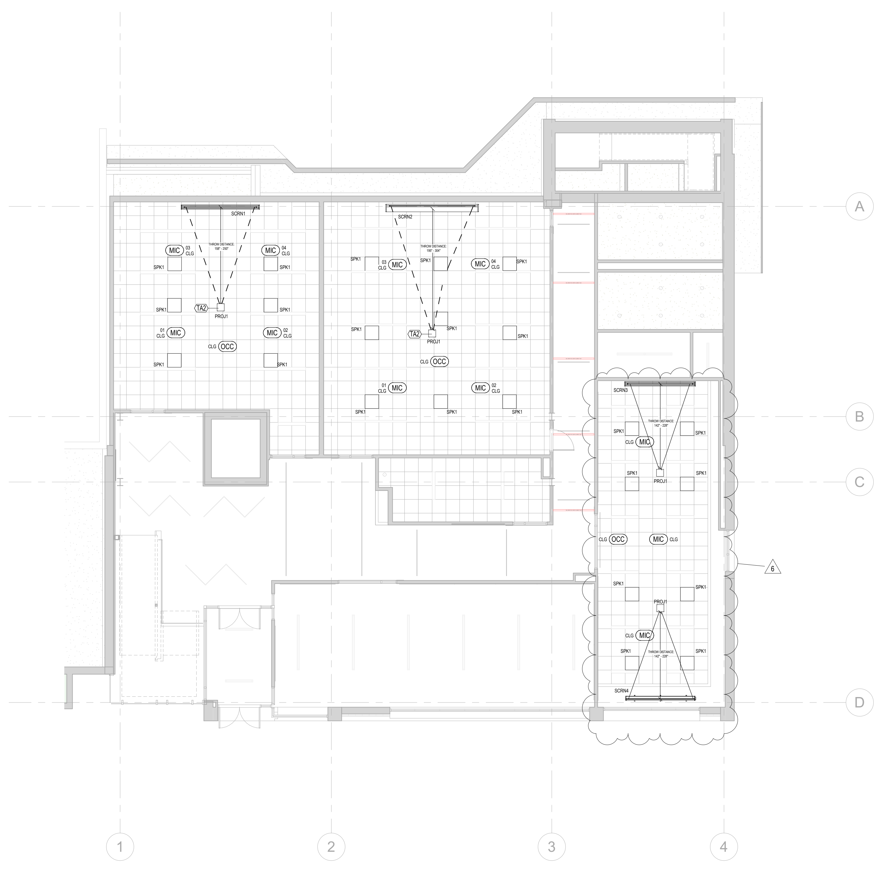
2 LEVEL 1 REFLECTED CEILING PLAN - AUDIOVISUAL 1/8" = 1'-0"
