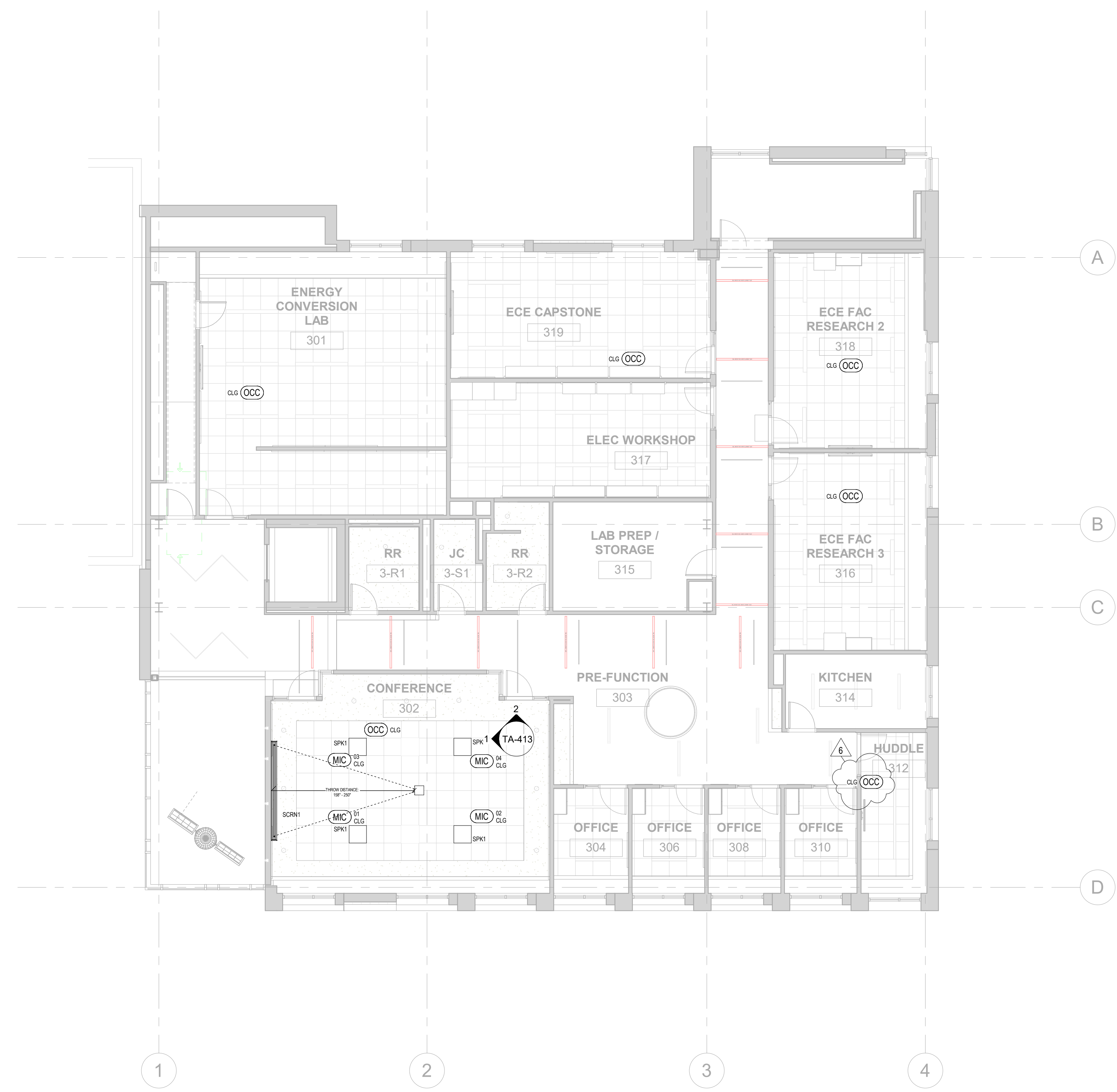
2 LEVEL 3 REFLECTED CEILING PLAN - AUDIOVISUAL 1/8" = 1'-0"
