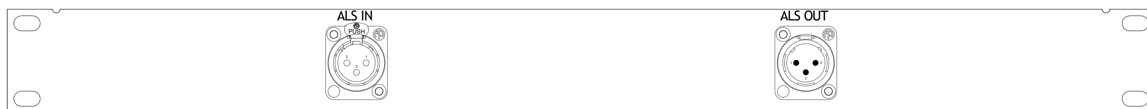
6 1RU AUDIO I/O PANEL - ASSISTED LISTENING SCALE: 6" = 1'-0"
